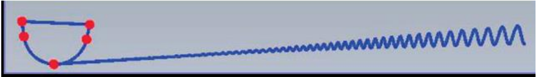
Sweeping vane tip profile along modulation curve.
